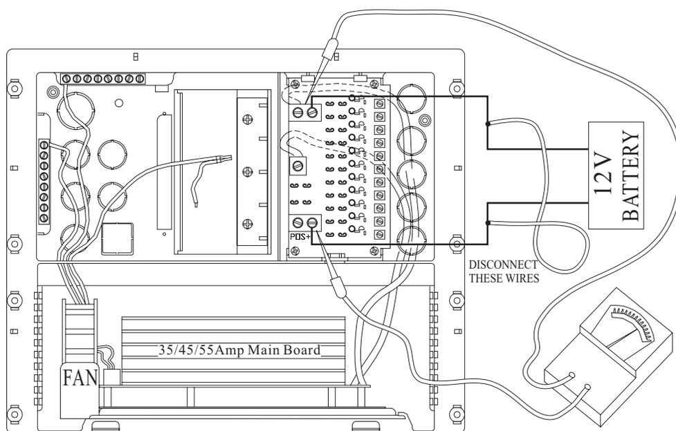
If converter output voltage reads 13.6 volts, but the battery is still not charging, check for an open automatic reset circuit breaker(if provided), or an open between the converter and distribution panel or an open wire between converter and RV Battery.
