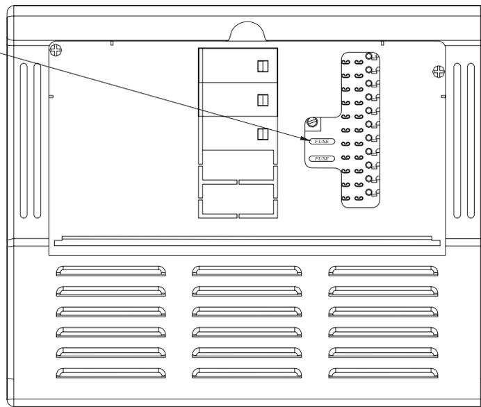
If fuse(s) are blown this means the RV Battery was accidentally connected in reverse either at the battery or at the converter. Connect properly then replace the fuse(s).
